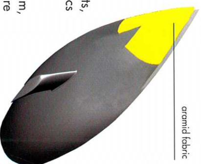
a sandwich laminate with PUR-foam core is used. The foam stability and the right material features are confirmed by independent certification agencies.
